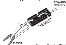
Figure 7: Line Tightener
