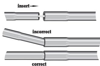
Figure 1: Correct Pole Assembly
