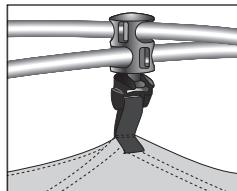
Figure 3: Quick Pitch Swivel Hub w/ H-clip (top view)
