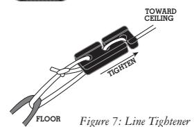
Figure 7: Line Tightener
