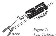
Figure 7: Line Tightener
