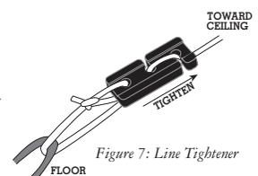
Figure 7: Line Tightener
