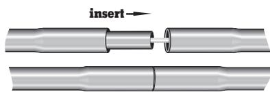
Figure 1: Correct Pole Assembly
