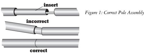
Figure 1: Correct Pole Assembly
