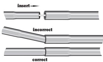
Figure 1: Correct Pole Assembly
