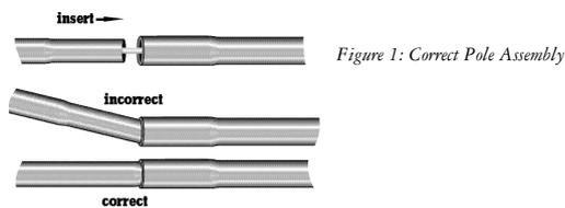
Figure 1: Correct Pole Assembly
