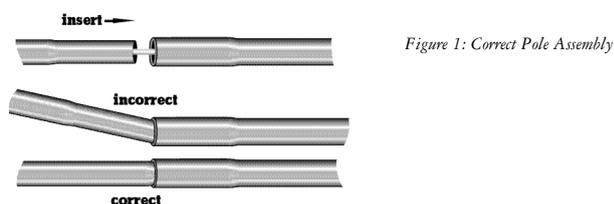
Figure 1: Correct Pole Assembly
