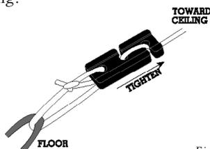
Figure 7: Line Tightener
