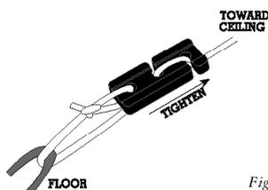
Figure 7: Line Tightener
