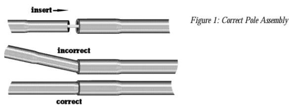
Figure 1: Correct Pole Assembly
