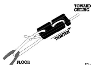
Figure 7: Line Tightener
