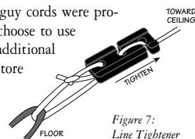
Figure 7: Line Tightener
