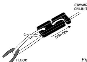
Figure 7: Line Tightener
