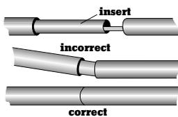
Figure 1: Correct Pole Assembly
