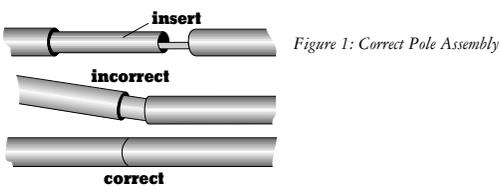
Figure 1: Correct Pole Assembly
